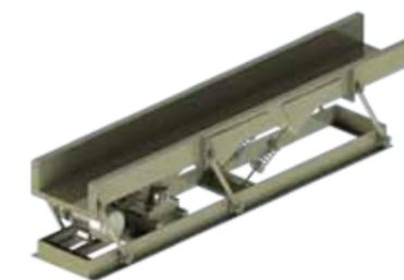
The HTV vibrating conveyors are designed as infeed conveyors for chippers. They can also be used as chip discharge conveyors for both shredders and chippers. Vibrating conveyors can be designed with a screening section and metal-free zone for mounting a metal detector or overbandmagnet
